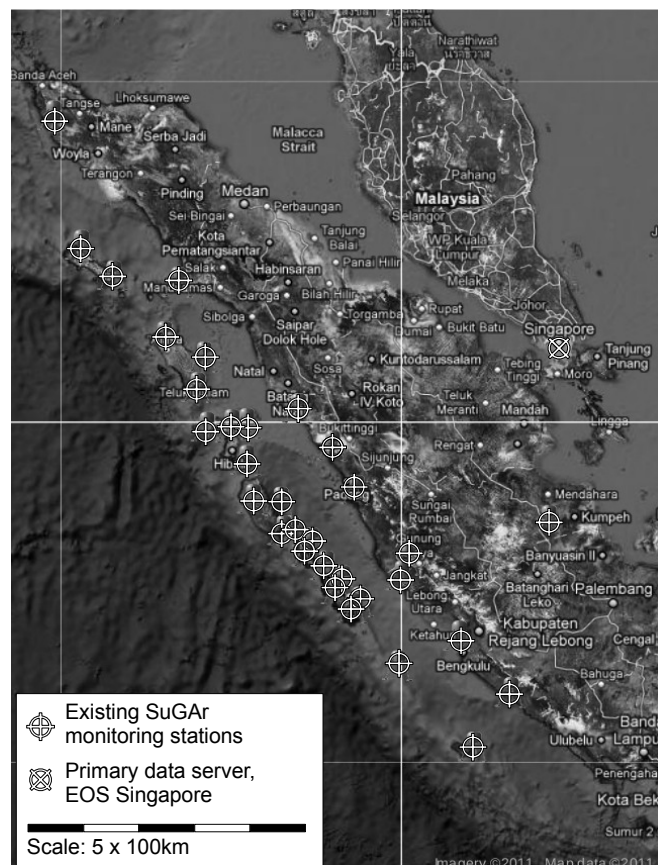
Fig. 1. The location of monitoring sites and central server for the Sumatran GPS array (SuGAR), spanning more than 1000km of known tectonic faults.
